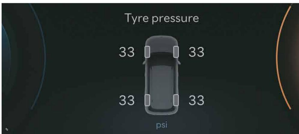
Tyre pressure monitoring system (TPMS) – Highline
