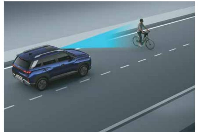
Forward Collision - Avoidance Assist - Cycle (FCA-Cyl)
