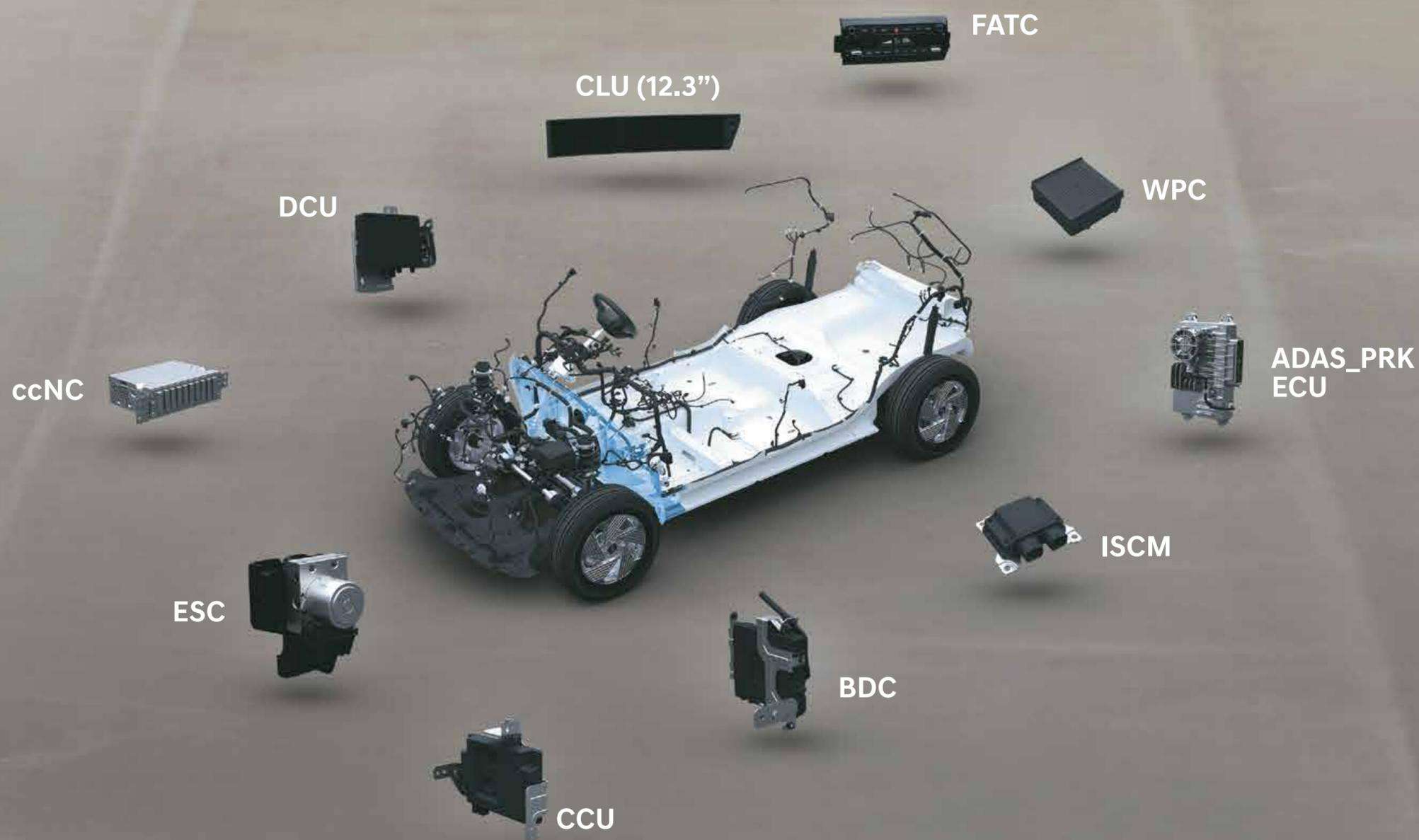
DCU - Data Connectivity Unit | CLU - Cluster | FATC - Fully Automatic Temperature Control | WPC - Wireless Power Charger
